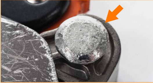
Closing pin completely worn.
