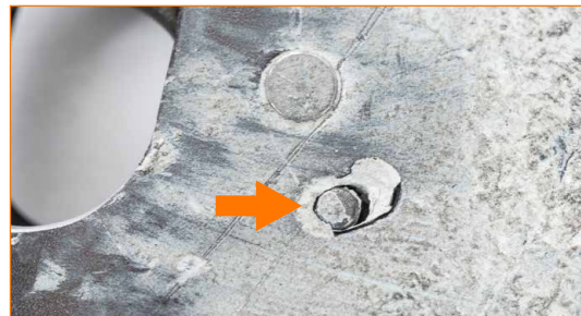
Deposits of hard material in the depression on the back of the device.
