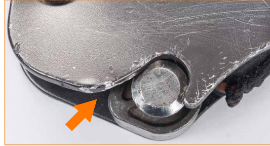
Movable side plate bent, no longer snaps onto closure pin.
