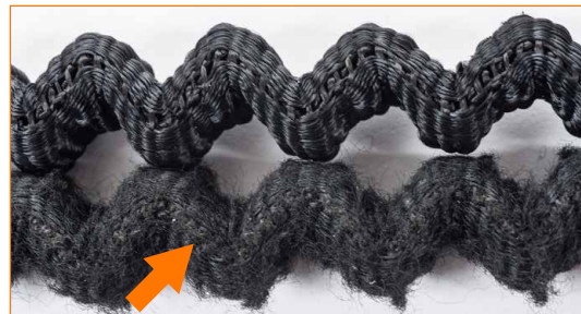
Elastic tape sling with clear evidence of wear (below). During the visual inspection the tape sling must be extended, so that hidden and potentially damaged parts can be examined.
