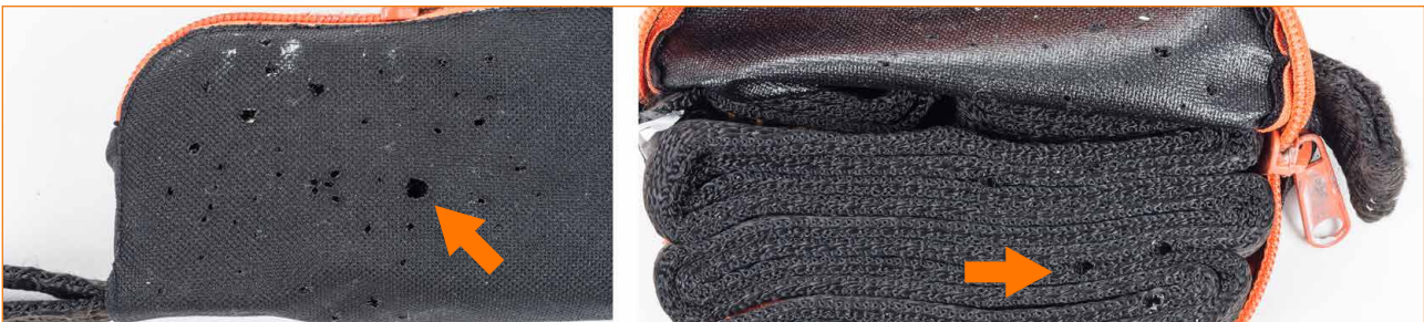
Case with signs of burning which are also present on energy absorber stored inside it.
