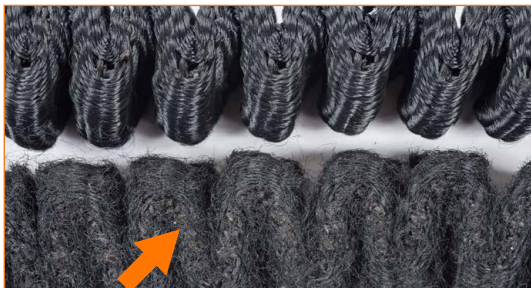
Elastic tape sling with clear evidence of wear (below). During the visual inspection the tape sling must be extended, so that hidden and potentially damaged parts can be examined.
