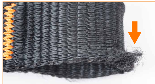
Elastic tape sling with end loop partially cut.
