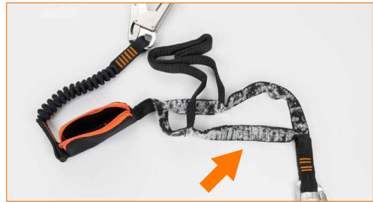
Energy absorber has been partially deployed.
