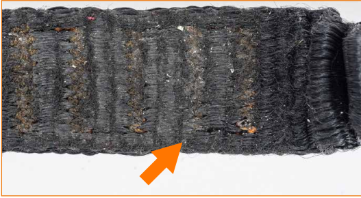
Safety stitching so dirty as to make visual inspection impossible.
