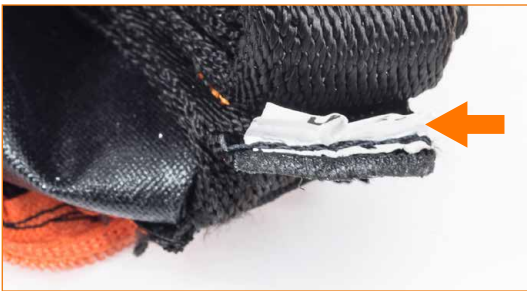
Missing labelling, label has been cut off.
