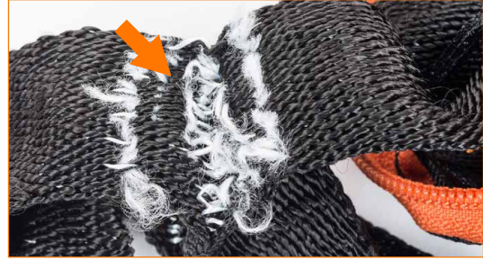
Energy absorber has been slightly deployed. The start of tearing is visible in the sling's stitching.
