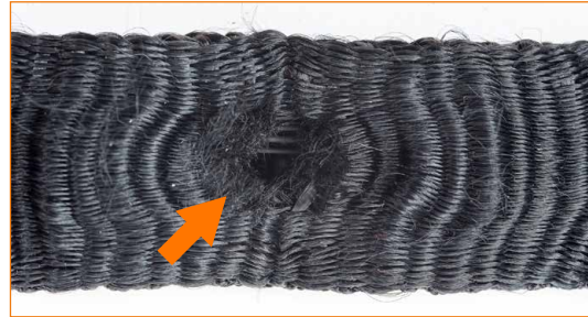
Elastic tape sling with clear cut in the loop.
